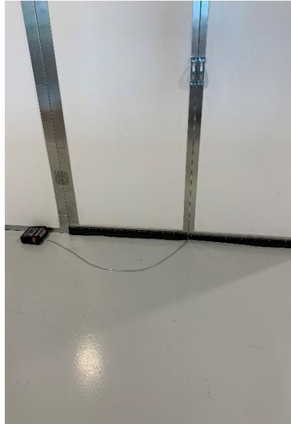
A 65-minute test was performed for both negative and positive pressure conditions. During each test, sixty 1-minute particle count samples were taken with a hold of 5 seconds between each sample. Pressure was measured about 5 minutes into the test to make sure a sufficient delta with the surrounding space was reached. At 30 minutes, the tester entered the room check the system, while also providing a rough simulation of a person entering the patient's room.
