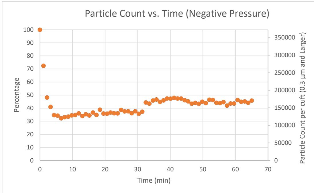
The chart below shows the key performance data collected for the negative pressure test. Note how quickly the environment reaches equilibrium as a result of the high number of air changes per hour.
